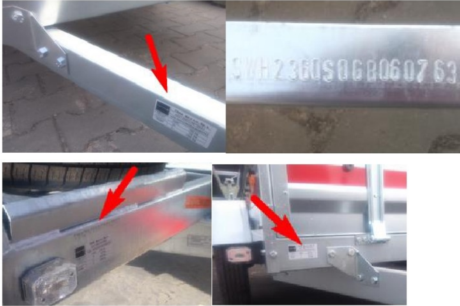
Fig. 1. Location of the trailer's nameplate
